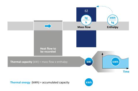
In addition to the above-mentioned variables, all "auxiliary variables" such as temperature, humidity, absolute pressure, enthalpy, density, velocity are available.
