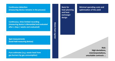
As shown in the diagram, each "level" has its justification, also with regard to the increasing costs from bottom to top. For a rough determination of the waste heat potential, it may be sufficient to measure temperature, humidity and flow rate using hand-held measuring devices.
